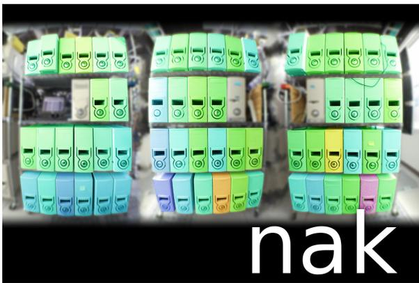
That's an actual photo of one of our clusters, NAK, tinted by **nodescape** as a real-time status display. Nodes are tinted from **blue-to-green-to-red** based on attribute values. As data ages (i.e., no new sensor readings are recorded), the tint increasingly dithers with **magenta**. A node with no data is tinted solid **magenta**.
